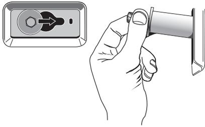
3. Once all 4 transport bolts are removed, discard bolt and spacers. Then pull the power cord through the opening of the rear panel and close the hole with the attached cap.
