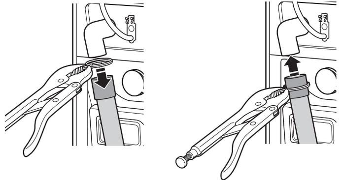
3. Once drain hose is in place, release pliers.
