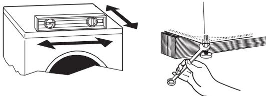
If the washer is against a wall, move the washer out slightly before tipping back. If the washer is not level, first prop the front with a wood block and adjust the feet as necessary; then prop the back and adjust feet as necessary. Repeat this step until washer is level.
