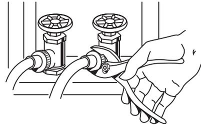
**NOTE:** Do not overtighten. Damage to the coupling can result.
