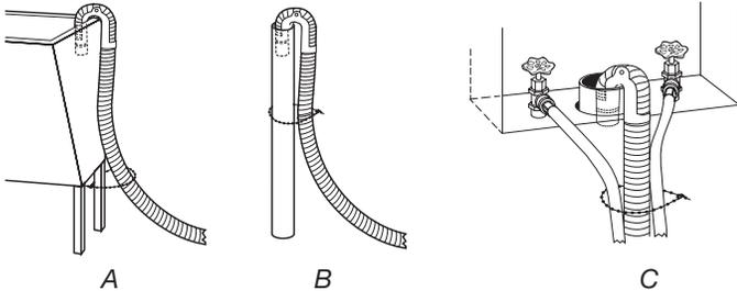
If the washer faucets and the drain standpipe are recessed (see illustration C), put the hooked end of the drain hose in the standpipe. Tightly wrap the beaded tie strap around the water inlet hoses and the drain hose.
